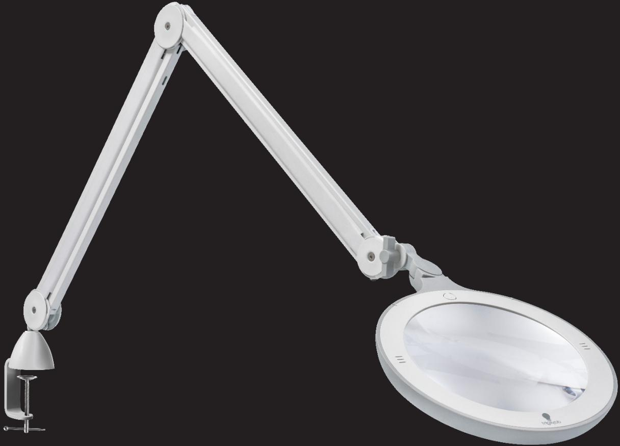
The Omega 7 is a modern, ergonomically designed magnifying lamp. It has a large 17.5cm, 3 dioptries (1.75X), lightweight acrylic lens and high power LEDs with 4 brightness level for clear viewing. The internal spring arm allows accurate positioning and lateral protections help you keep it clean. The aesthetically pleasing white and grey finish fits perfectly within any professional environment.
